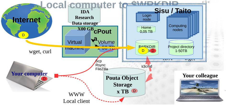
2. Process your data at CSC and backup intermediate steps to object storage Sisu / Taito **IDA** Login Research Internet node Data storage Computing X00 GBcPout Home nodes 0.05 TB /olume Virtual 1-50 TB Project directory machine 1-50TB s3cmd Your computer Your colleague **Pouta Object** Storage x TB WWW Local client
